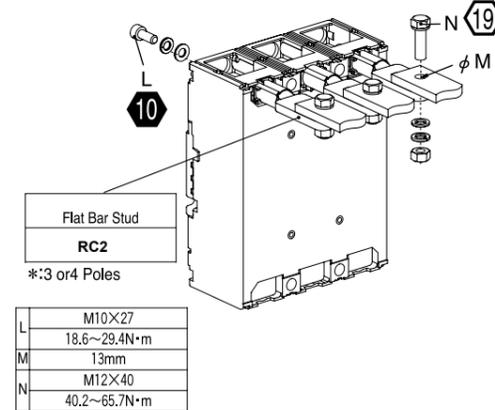
8 Conductor Connection Procedure for PM
