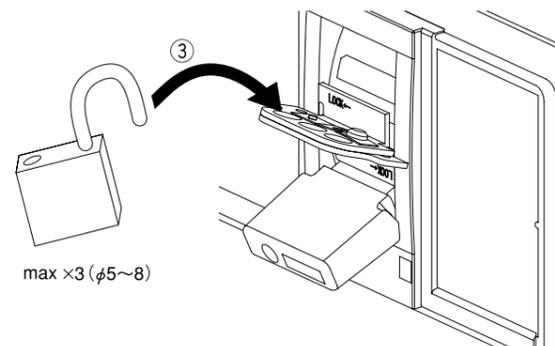
•Handle holder/ lock can be fitted in any position of | (ON) and ○(OFF).
