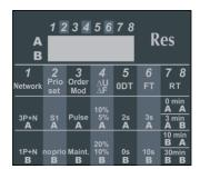
Programming through DIP switches is done using the 8 DIP switches on the front of the controller. Each DIP switch has positions A & B, by default all DIP switches are in position A.
